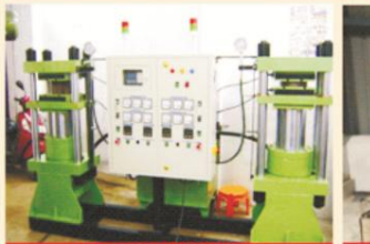
80T PLC OPERATED
